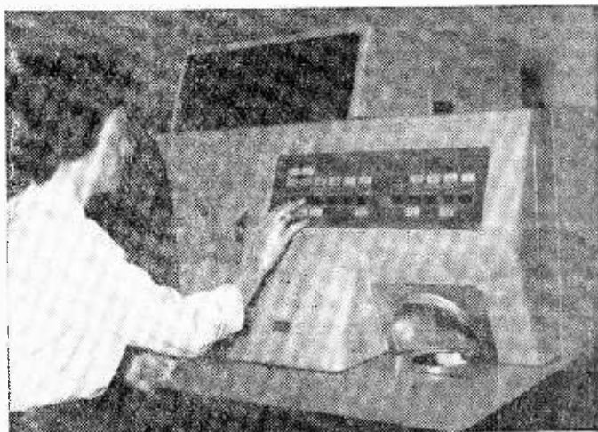
An operator actuating the controls of the reading console of the Solartron ERA (Electronic Reading Automaton). The tally roll on the right-hand side has been read by the machine.
